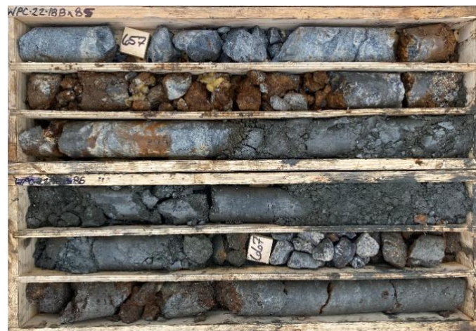
Photo 4. WPC22-18: 147.2-248.9 – 101.7 meters Portion of WPC22-18 showing high-grade massive galena in a dolomite matrix along with thick zones of intermingled massive pyrite
