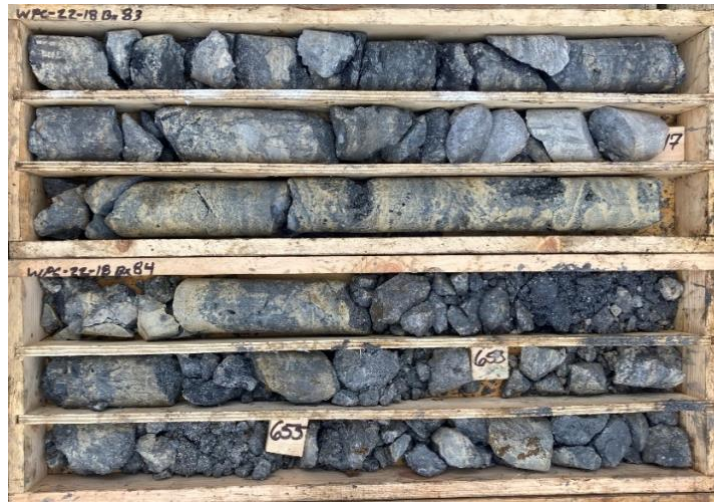
Photo 3. WPC22:-18 147.2-248.9 – 101.7 meters Portion of WPC22-18 showing lead-dominant mineralization with abundant argentiferous galena in a matrix of dolomite
