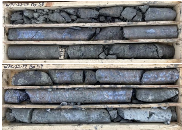
Photo 1. WPC22-17: 125.5-172.5 - 47.0 meters Portion of WPC22-17 showing massive reddish-brown sphalerite intergrown with argentiferous galena
