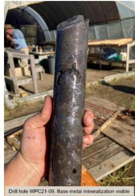
Figure 2: Cross-section of 2021 high-grade intercept and historical drilling. Photo: WPC21-09 drill core with visible mineralization of sphalerite and argentiferous galena
